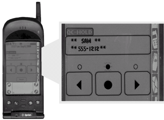
Figure 2. A three-button design allows users to respond with button presses rather than by speaking aloud.
